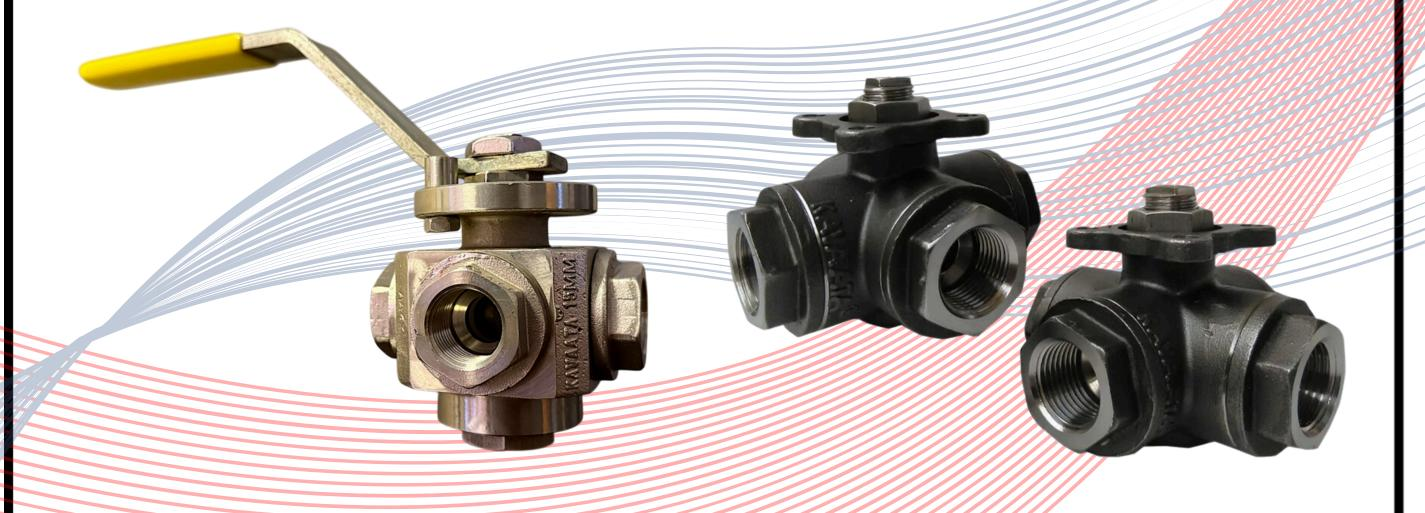
4 Way Ball Valves are offered with L-L port or Double L Port and are manufactured with screwed ends. These valves are used when two right-angle diversions have to be done using one single valve. These valves will have two inlets and two outlets at any given time. The balls inside the valve are precisely machined to achieve this objective.
