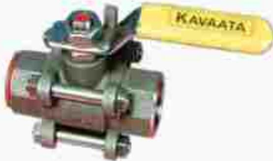
Kavaata Screwed End Investment Cast Ball Valves are designed and manufactured as per **BS5351/ISO17292** or **API 6D** standards. The material of construction generally offered are **ASTM A216 Gr WCB (CS)**, **ASTM A351 Gr CF8 (SS304)** and **ASTM A351 Gr CF8M (SS316)**.
