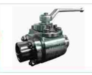
Metal seated Ball Valves are preferred when the operating temperature is typically above 250 deg C and upto 600 deg C, where the soft seats fail. The ball made of SS304/SS316 is either coated with Nickel (by Electroless Nickel Plating) or hard faced with Stellite or coated with Chrome Carbide (HVOF) depending upon the operating temperature and pressure. The matching metal seats are also hard faced or HVOF coated.
