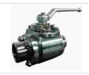
Metal seated Ball Valves are preferred when the operating temperature is typically above 250 deg C and upto 600 deg C, where the soft seats fall. The ball made of \$\$304/\$\$S316 is either coated with Nickel (by Electroless Nickel Plating) or hard faced with Stellite or coated with Chrome Carbide (HVOF) depending upon the operating temperature and pressure. The matching metal seats are also hard faced or HVOF coated.
