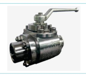
Metal seated Ball Valves are preferred when the operating temperature is typically above 250 deg C and upto 600 deg C, where the soft seats fail. The ball made of **SS304/** SS316 is either coated with Nickel (by **Electroless Nickel Plating**) or hard faced with **Stellite** or coated with **Chrome Carbide** (HVOF) depending upon the operating temperature and pressure. The matching metal seats are also hard faced or HVOF coated.
