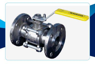
Kavaata Flanged End Ball Valves are made from Investment Castings, designed & manufactured as per ISO 17292 / API6D standards. The material of construction generally offered are ASTM A216 Gr WCB (CS), ASTM A351 Gr CF8 (SS304) & ASTM A351 Gr CF8M (SS316).
