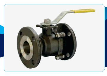
Flanged End two piece design Ball Valve are economical & less prone to leakages & are by far most commonly used Ball Valves in the industry. These Ball Valves are available in ASA Class 150# & are tested as per Fire safe test standards such as API 607 VI edition / ISO 10497:2010.
